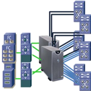
Figure 2. Cloud unit of storage, network, and compute showing “port explosion” phenomena
